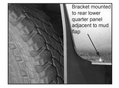
Attach with 10-24 x 1-1/2" truss head screws with flat washers and
