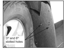
D. Install #10 x 1-1/4" self-drilling hex screw with washer at upper mounting hole.
