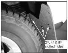
D. Verify mud flap is level then install #10 x 1-1/4" self-drilling hex screw with washer at upper mounting hole.
