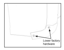
B. Install mud flaps with (2) 7 mm hex screws through 3<sup>rd</sup> and 6<sup>th</sup> slotted holes into newly free holes in wheel well. Leave screws loose for now.
