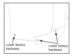
B. Install mud flaps with (3) 7 mm hex screws through 2<sup>nd</sup>, 4<sup>th</sup> and 5<sup>th</sup> slotted holes into newly free holes in wheel well. Leave screws loose for now.
