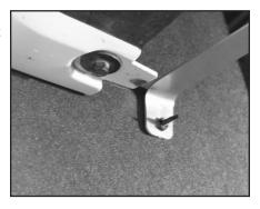
E. With stabilizing bracket attached to mud flap, adjust stabilizing bracket until enough clearance is provided in wheel well.
