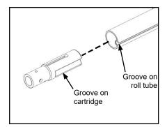
B. Use small groove on cartridge as guide to measure along side of roll tube and mark 5" in from end of cartridge, then drill 13/32" hole through first layer of roll tube.
