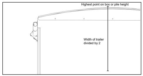
B. At previously recorded height, center mounting plate horizontally then mark hole locations on mounting plate.
