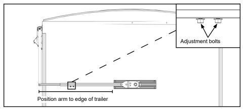
D. Torque 3/8" x 1" adjustment bolts to 32 ft-lbs.
