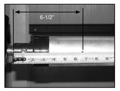
D. Drill 5/16" hole through roll tube and first wall of cartridge inside of tube.
