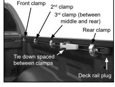
D. Place side rail between clamps and inside lip of box until it rests on deck rail. Use standard instructions for correct height and position of side rail.
