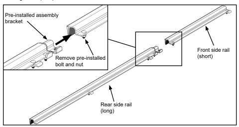
D. Attach short side rail (front) to assembly bracket with previously removed 1/4" x 3/4" carriage bolt and nylock hex nut. Align side rails then tighten with 7/16" wrench.
