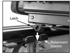
D. Attach safety straps to brackets on each side.
