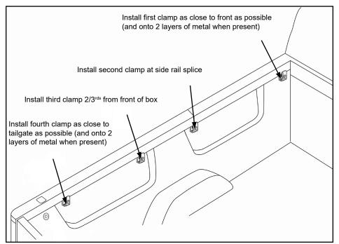
**NOTE:** For trucks with electric tailgates, typically side rail must be installed slightly higher to eliminate interference.
