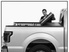
C. Always ensure hooks and latches fully engage catches and side rails. Close tailgate.
