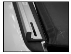
B. Lift rail until slotted hole is accessible from bottom. Route knot in cord under and through slotted hole, then drop clamp plate into stake pocket and lower rail.
