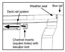
**NOTE:** Position tie downs as desired between brackets. After installing cover, ensure cover components do not contact tie downs. Adjust tie downs as needed.
