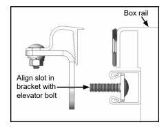
G. Ensure side rail is level and secure front and middle bracket with 1/4" serrated nut.
