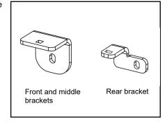
A. Align square holes in front and middle brackets with holes in side rail. Secure with 1/4" x 3/4" bolts, flat washers, lock washers and nuts, then tighten.
