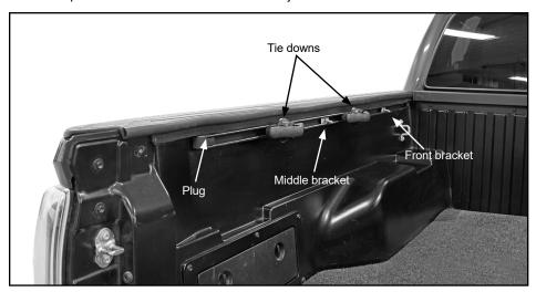
E. Reinsert deck rail system plug at end of channel near tailgate.
