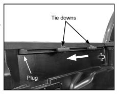
C. Use 10 mm socket with ratchet to remove 6 mm bolt near rear of truck. Save 6 mm bolt for reuse in Step 3H.
