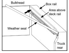
**NOTE:** Ensure top of seal is aligned with top of box rail.
