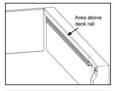
B. Peel small segment of protective backing from one end of "D" weather seal. At rear of truck, align top of weather seal with top of box rail then adhere weather seal segment without backing to vertical surface above deck rail system.
