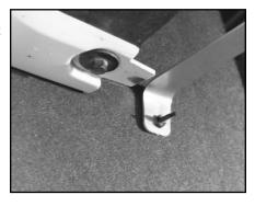
E. With stabilizing bracket attached to mud flap, adjust until enough clearance is provided in wheel well.
