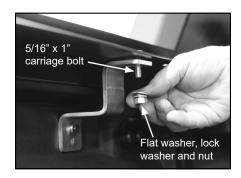
B. Push side rail tight against box rail to compress seal. Ensure entire seal is completely compressed then fully tighten nut.
