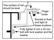
B. Install brackets at middle and rear of side rail. While side rail is level and correct height, ensure bracket is flush and tight with box wall and side rail.
