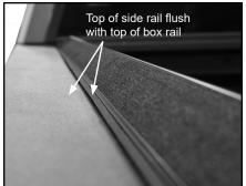
B. Clean inside edge of box rail with alcohol pad. Peel protective tape from seal. Position side rail tight to front of box and flush with box rail. Working from front of box to rear, adhere side rail to inside edge of box rail.
