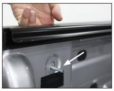
D. Place other half of clamp over bolt and turn nut finger tight.
