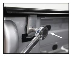
ALTERNATE LOCATION OF LONG CLAMP - only if stake pocket is not available, use shim at this location. Even if stake pocket is utilized with an accessory, remove it and check for space. Usually the long clamp will install down in the pocket and still allow the accessory to be remounted.
