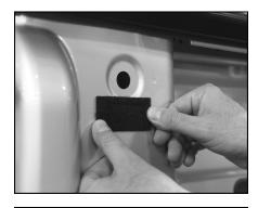
B. At top of rear stake pocket, lower back half of long clamp with fish wire and carriage bolt down into pocket.
