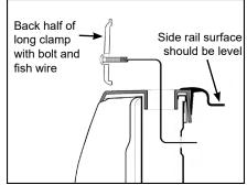
C. Using fish wire, align and pull bolt through hole on inside wall of box and hold.
