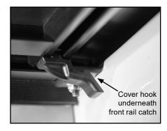
C. With cover hooks engaged underneath front catches, lower cover to engage latches in retainment brackets on each side.
