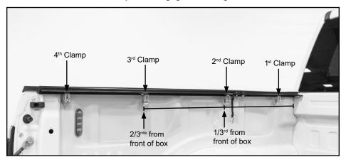
**NOTE:** For trucks with electric tailgates, typically side rail must be installed slightly higher to eliminate interference.
