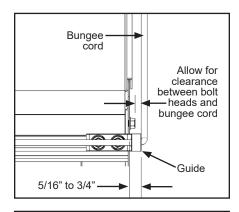
B. Use guide as template to drill (2) 5/16" holes. Fasten guide with 3/8" x 1" self-threading bolt in each hole.
