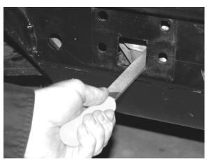
**Step 1** - If vehicle is equipped with 1<sup>1</sup>/<sub>4</sub>" receiver, remove and set aside. With flat file, file corner radius square on all four corners of existing opening until new 1<sup>1</sup>/<sub>2</sub>" receiver fits through.
