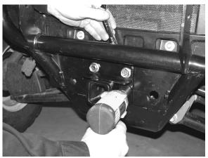
**Step 3** - Use wrench to hold nut on back and tighten the four bolts. When done torque all bolts to 75 foot lbs. Check torque periodically and retorque if needed.
