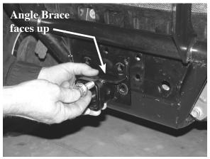
**Step 2 -** Place new receiver over opening with angle brace facing up (see photo). Insert four bolts from the front. Turn nuts on from backside.
