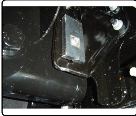
4. Raise hitch into position and push bolts out. Attach M12-1.75 hex flange nut to bottom bolt on each side. Re-attach (2) nuts removed in STEP 2 to top bolt on each side.
