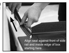
IMPORTANT: Ensure raised portion of seal is against inside edge of box while unraised portion is toward cab.
