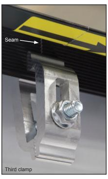
E: Place final fifth clamp at rear of box as close to tailgate as possible where 2 layers of metal are present. Always make sure clamp teeth engage grooves on rail. Repeat Step 1 to install rail on opposite side. **When done, make sure all clamps are torqued to 20 ft-lbs.**
