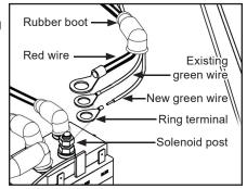
NOTE: If system runs backwards, switch piggy back terminals on solenoid.
