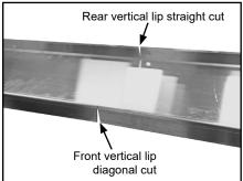
F. Place metal filler on box and press down on ends to angle metal filler at notches until it meets edge of box.
