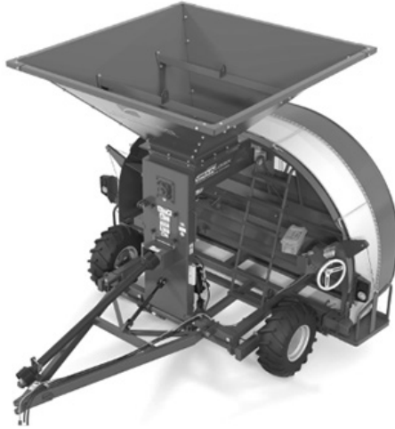
Grain bag loader without access platform
