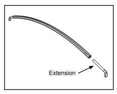
C. Raise bow up to proper height (1-1/2" above end cap vertical to box) and hold. Drill 5/16" hole through one side of bow (ensure location will not cause bolt head to rub on tarp) and bow extension. Turn a 3/8" self threading bolt into holes and tighten.
