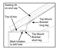
C. Drill 3/8" hole through location marked on top of box and insert bolt, flat washer, lock washer and tighten with nut.
