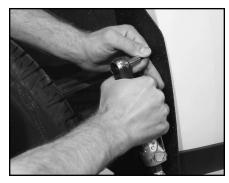
**NOTE:** Use sufficient screws, kit provides 6 per mud flap or 4 if the stabilizing bracket is installed.
