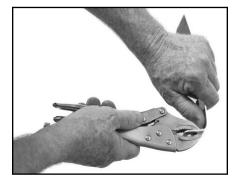
C. Using stabilizing bracket as guide use angled screwdriver with self-drilling screw to carefully drill a hole in mud flap, then remove screw.
