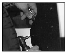
E. With stabilizing bracket attached to mud flap, adjust stabilizing bracket until enough clearance is provided in wheel well.
