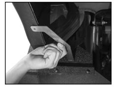
B. Use locking pliers to bend stabilizing bracket as needed.
