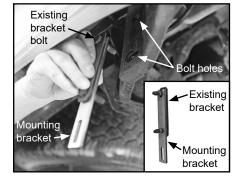
D. Secure with nuts and tighten with ratchet and 15 mm socket until snug, but not completely tight.
