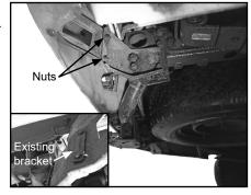
C. Insert existing bracket bolts through mounting bracket, then reinsert bolt into bolt holes.
