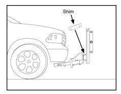
G. If push frame leans away from front of vehicle, remove lower bolts and insert one or two shims at bottom and reinsert bolts.
