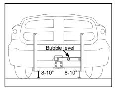
E. Check push frame for vertical plumb.
