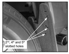
D. Verify mud flap is level then install #10 x 1-1/4" self-drilling hex screw with washer at pinhole guide. Secure with nylon hex nut.
