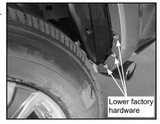
B. Install mud flap with (3) #14 x 1" Phillips head hex screws through 2<sup>nd</sup>, 4<sup>th</sup> and 5<sup>th</sup> slotted holes into newly free holes in wheel well. Leave screws loose for now.
