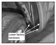
B. Install mud flap with (3) #14 x 1" Phillips head hex screws through 1st, 3rd and inner most slotted holes into newly free holes in wheel well. Leave screws loose for now.
