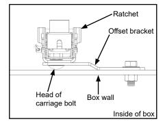
A. Insert 3/8" carriage bolts through slotted bracket holes and ratchet. Secure bolts with flat washer, lock washer and nut then tighten with 9/16" wrench.
