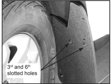
C. Level mud flap while adjusting placement to obtain best fit then tighten screws to hold in place.
