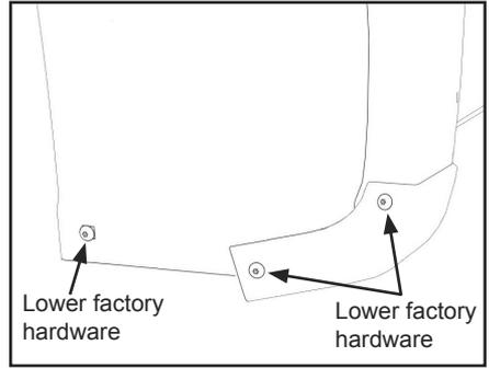
B. Install mud flaps with (3) 7 mm hex screws through 2<sup>nd</sup>, 4<sup>th</sup> and 5<sup>th</sup> slotted holes into newly free holes in wheel well. Leave screws loose for now.
