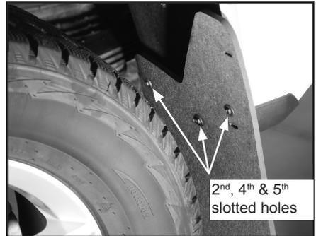
D. Verify mud flap is level then install #10 x 1-1/4" self-drilling hex screw with washer at upper mounting hole.
