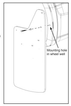
D. Install (3) #10 x 1-1/4" self-drilling hex screws with washers at remaining slotted mounting holes and tighten screws.
