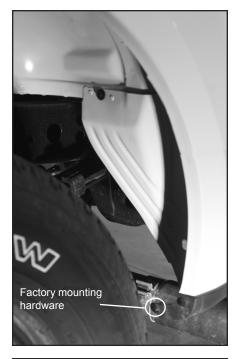
B. Install 10-24 x 1-1/2" truss head screw with washer at 4<sup>th</sup> slotted mounting hole from top. Secure with nut.
