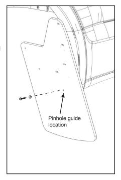
G. Verify mud flap is level then install (2) #10 x 1-1/4" self-drilling hex screws with washers at remaining pinhole guides and (1) #10 x 1-1/4" self-drilling hex screw with washer at upper mounting hole. Ensure screws contact metal backing as much as possible
