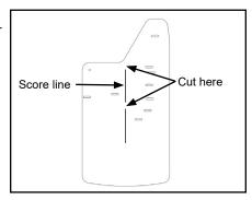
B. Using adjacent image as a guide, remove plastic insert with cutting tool and (3) lower factory screws with 10 mm socket.
