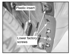
C. Position mud flap with the inner half behind wheel well.
